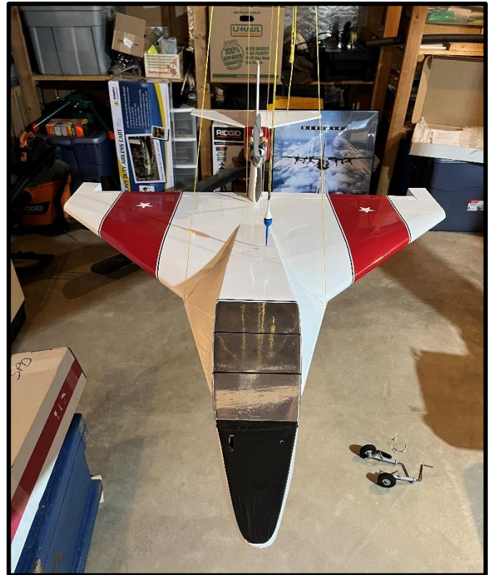
Using a Vanessa Rig to balance the Northstar
